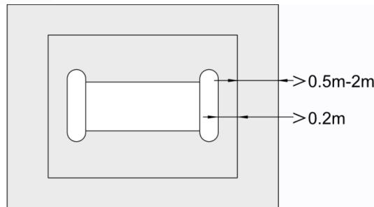
Note: Make the Receiving Coil (RX) away from the interference source. Make sure the interference level displayed on the environment inspection indicator is less than 2.
